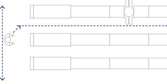
In the event of yarn break, Individual spindle light indicator guides the operator directly to the spindles.
