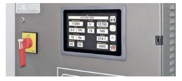
This system includes axial displacement, realized by the electronic thread-guide control, which allows the yarn distribution over package edges, to obtain a "Customized" Package design. The bunching length is settable by the PC, as well as its position on the package tube. The working parameters can be varied flexibly, there are no more pre-set ranges, this allows our customers to obtain the best results, both in terms of working speed and package formation.
