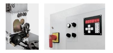
Allowing customers to set all working parameters via PC, machine set-up time is strongly decreased, by introducing a simple and direct way to change any setting. This system allows to reduce the number of operators for each machine, and to change settings continuously and not "step by step", as in the mechanical version, allowing customers to try any parameters combination, in order to obtain the best results.
