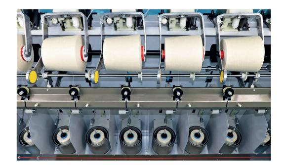
The use of the bigger diameter spindle involves: lower needs of work force, less package doffing is necessary at a certain package weight, lower number of joints in the final package.
