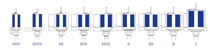
The use of the smaller diameter spindle involves: lower energy consumption, less energy per kilos of twisted yarn produced, higher twisting speed and higher productivity, lower twisting tension and better quality of twisted yarns, less noise at the same speed.
