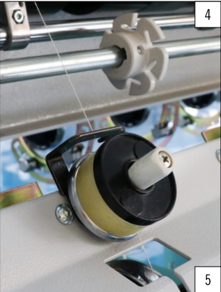
Yarn reserve (4) As required by down stream process like weaving to enhance the running efficiency of the process, the yarn reserve can be installed for uniform tail end preparation.
